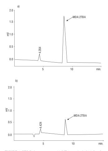
FIGURE 1. HPLC chromatograms: (a) MDA standard, (b) infant formula. Column: Hypersil<sup>®</sup> BDS C18 (250 × 4.6 mm, d<sub>p</sub> 5  $\mu$ m), mobile phase: 5 mmol/L sodium phosphate buffer (pH 7.0) and acetonitrile (85:15, v/v). Flow rate: 07 mL/min. Detection: 532 nm.
